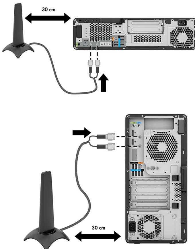
For best performance, place the antenna on either side of the computer where it has the clearest line-of-sight to the access point or router. The recommended distance is more than 30 cm from the computer. Avoid placing the antenna in front, behind, or on top of the computer because of the risk of noise interference.
