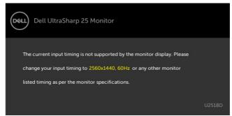
This means that the monitor cannot synchronize with the signal that it is receiving from the computer. See Monitor Specifications for the Horizontal and Vertical frequency ranges addressable by this monitor. Recommended mode is  $2560 \times 1440$ .
